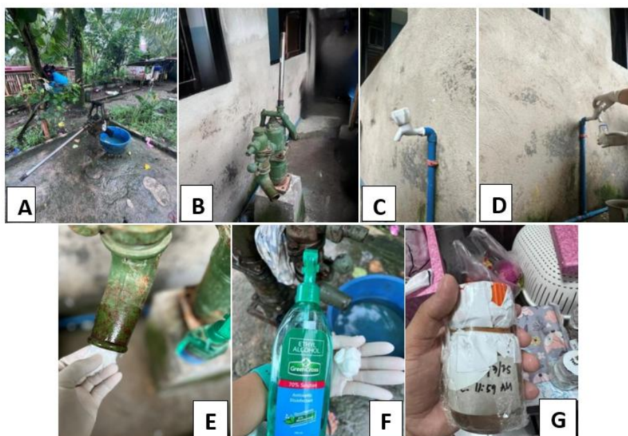
Figure 3. Groundwater sampling sites and water sample collection procedures. (A–C) The three deep well sampling sites (DW1, DW2, and DW3) selected for physicochemical and microbiological analyses. (D–F) Preparation of the sampling outlets before water collection, including removal of the cloth filter, outlet sanitization with 70% alcohol, and flushing for approximately three minutes to remove stagnant water and reduce the risk of sample contamination. (G) Sterile 100-mL sampling bottles and an insulated cooler used for the preservation and transport of water samples to the microbiology laboratory.
