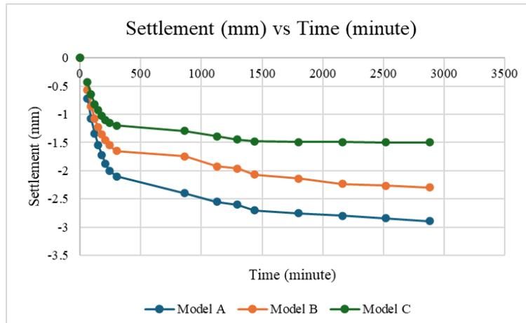
**Figure 6.** Settlement vs time graph for Model A, Model B, and Model C.
