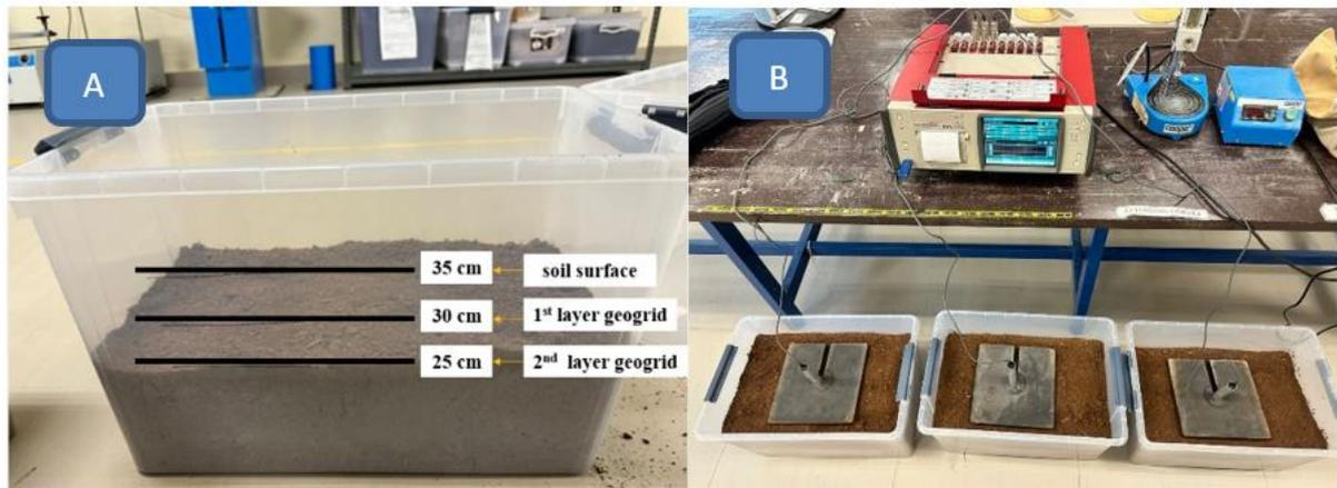
**Figure 4.** (a) Height placement of two-layer bamboo geogrid; (b) Setup with LVDT, data logger, and 15 kg loading plate.
