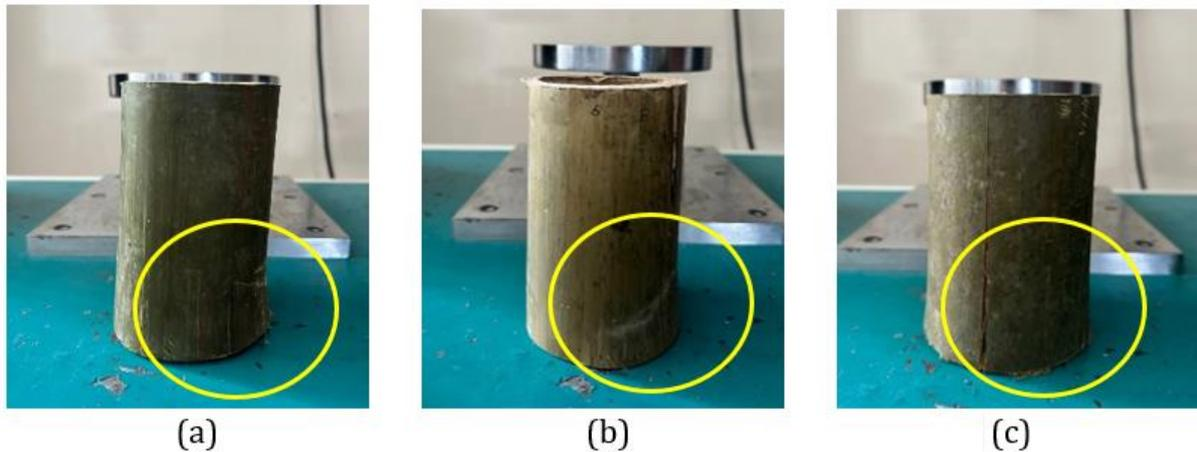
**Figure 5.** Cracks in Bamboo After CS Test (in yellow) (a) Bamboo A; (b) Bamboo B; (c) Bamboo C
