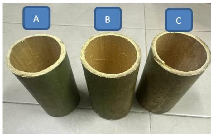
**Figure 2.** Bamboo samples A, B, and C, each with a height of 150 mm.
