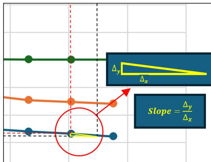
**Figure 7.** Triangular method for the slope of settlement curves.
