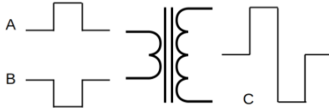
Figure 3. Operating principle of the box signal inverter: A and B (the input square wave signal consist of two square waves with a 180^\circ phase different), and C (output signal voltage).
