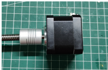
Figure 9 Actuator design: (a) NEMA 17 stepper motor module.
