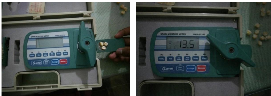
Figure 2. Measurement of corn kernel moisture content using the standard grain moisture meter.
