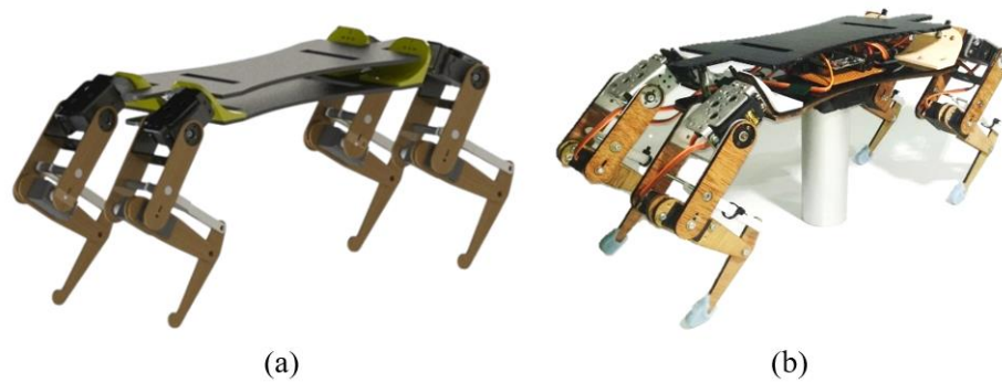
Figure 1. Design and prototype of the cat robot. (a) 3D model of computer-aided design; (b) Resulted prototype.
